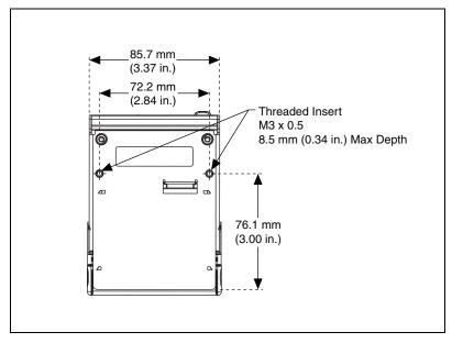
Figure 6. Module Dimensions in Millimeters (Inches)
